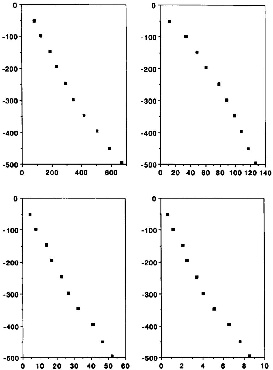
**Figure 2** Cumulative color change ( $\Delta E$  units) for curcumin passive sampler vs cumulative ambient concentration of ozone (upper left), NO<sub>2</sub> (upper right), PAN (lower left) and PPN (lower right)
