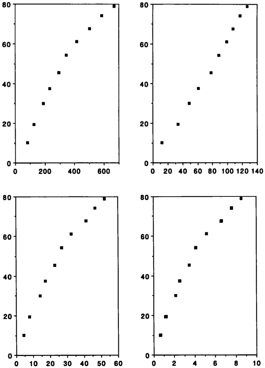
**Figure 5** Cumulative color change ( $\Delta E$  units) for 1-methylperimidinium passive sampler vs cumulative ambient concentration of ozone (upper left),  $\text{NO}_2$  (upper right), PAN (lower left) and PPN (lower right)
