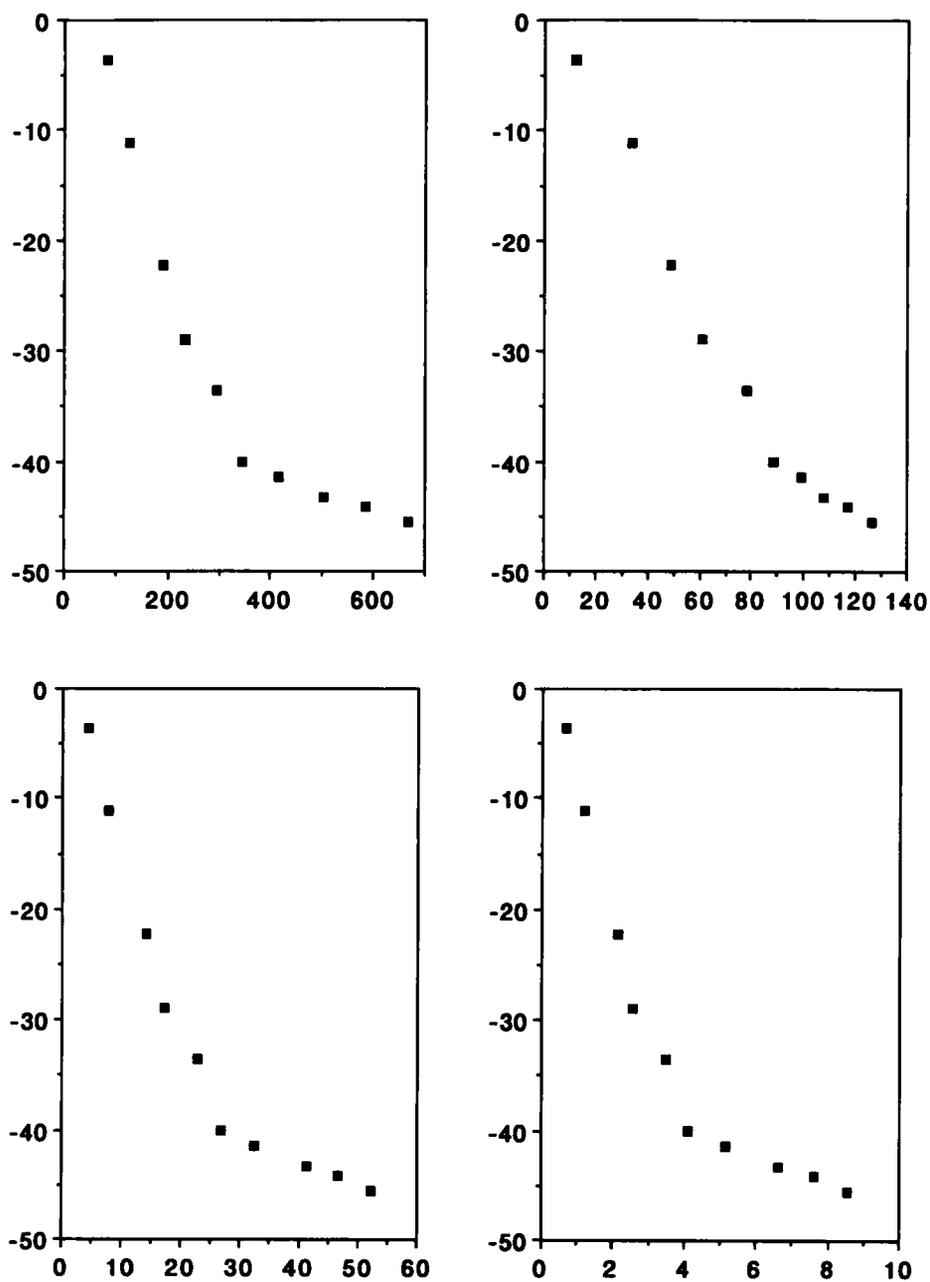
**Figure 3** Cumulative color change ( $\Delta E$  units) for Disperse Blue 3 passive sampler vs cumulative ambient concentration of ozone (upper left),  $\text{NO}_2$  (upper right), PAN (lower left) and PPN (lower right)
