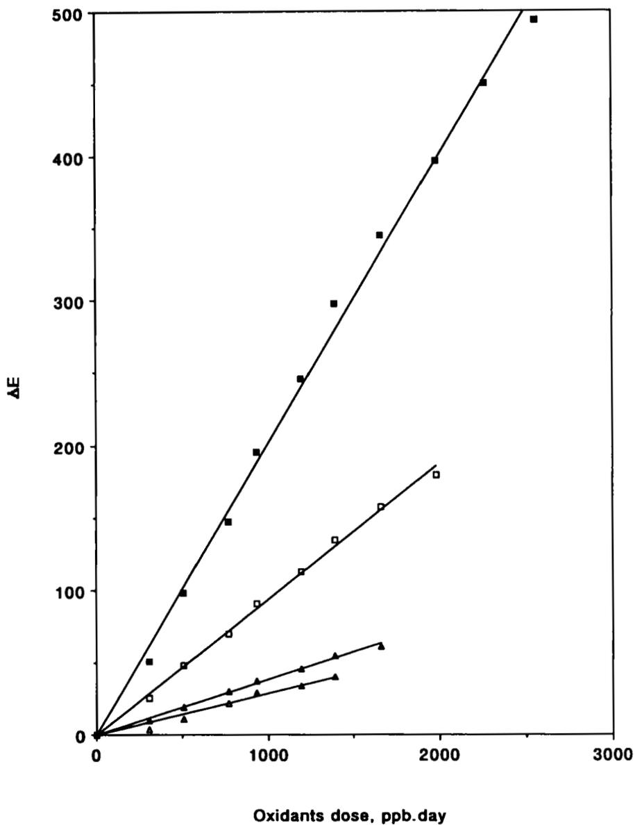
**Figure 6** Cumulative color change ( $\Delta E$  units) versus cumulative total oxidants dose ( $\text{O}_3 + \text{NO}_2 + \text{PAN} + \text{PPN}$ ) for curcumin (top, solid squares), phenoxazine (open squares), 1-methylperimidine (solid triangles) and Disperse Blue 3 (bottom, open triangles). Linear regression parameters are given in Table 2.
