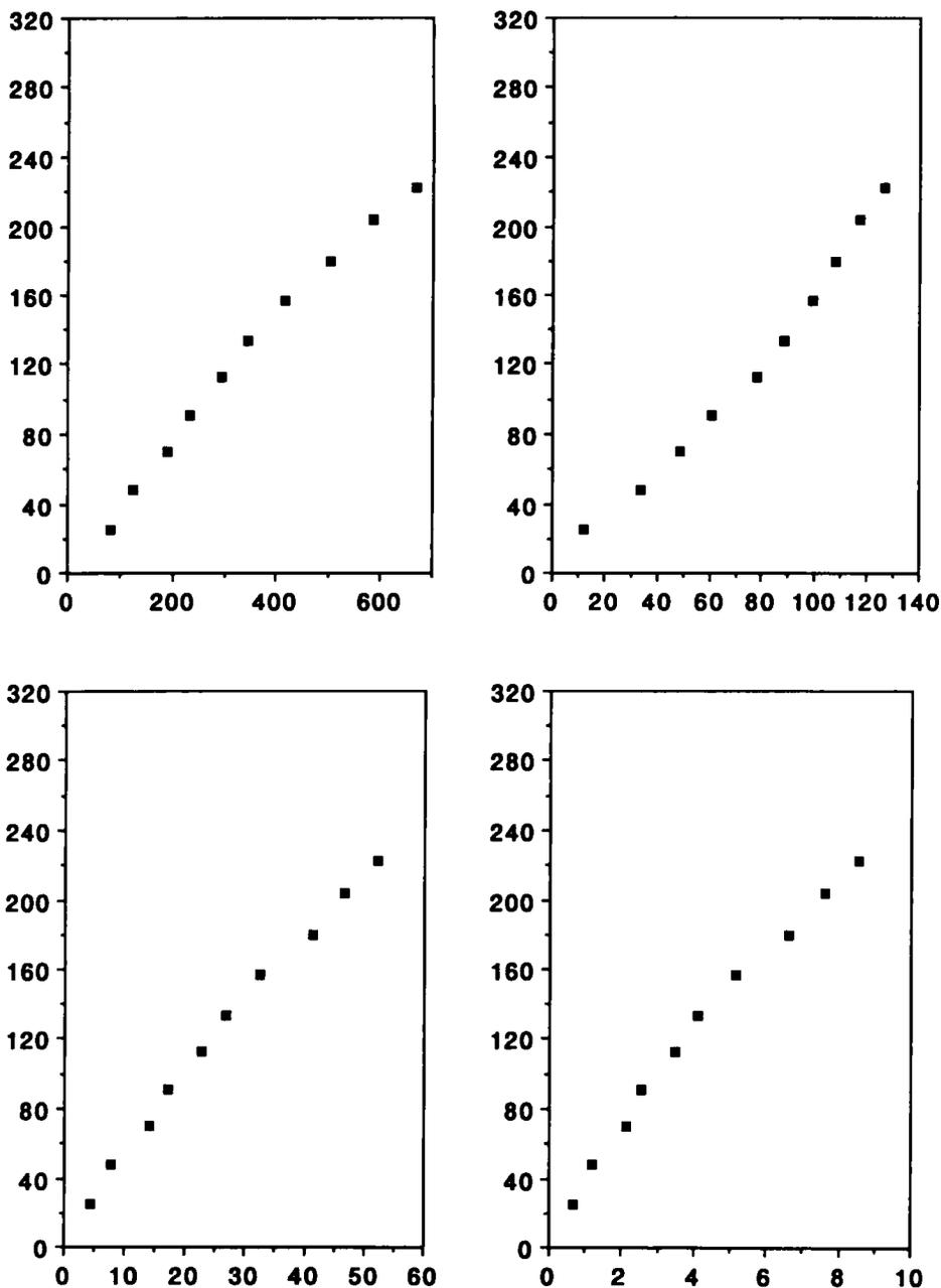
**Figure 4** Cumulative color change ( $\Delta E$  units) for phenoxazine passive sampler vs cumulative ambient concentration of ozone (upper left), NO<sub>2</sub> (upper right), PAN (lower left) and PPN (lower right)
